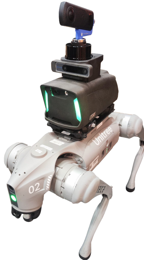
The scanner on this mechanical dog helps the project team track work progress
